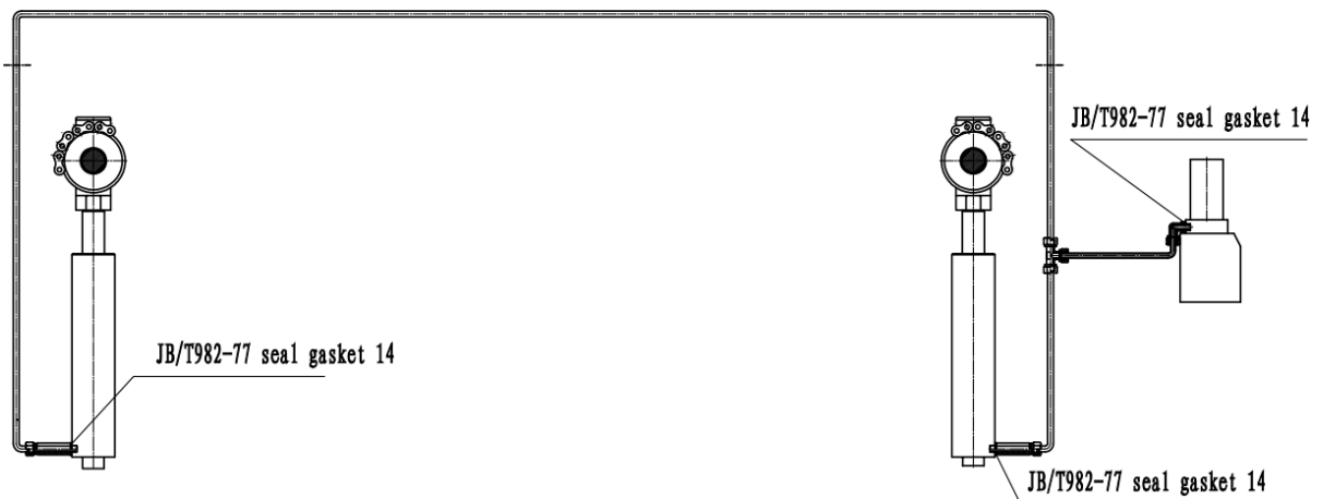
Diagram of hydraulic line of floor-plate 2-post lift
